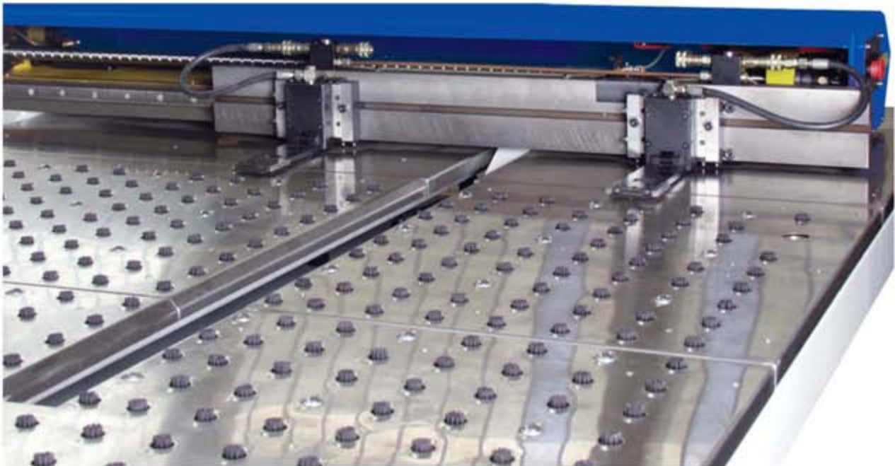
HTP 30322 table and hydraulic / pneumatic sheet clamps
